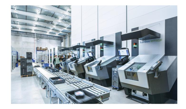
Solution #1: Vertical Buffer Module Kardex Compact Buffer with the order fulfillment system Kardex Frame Pick System
