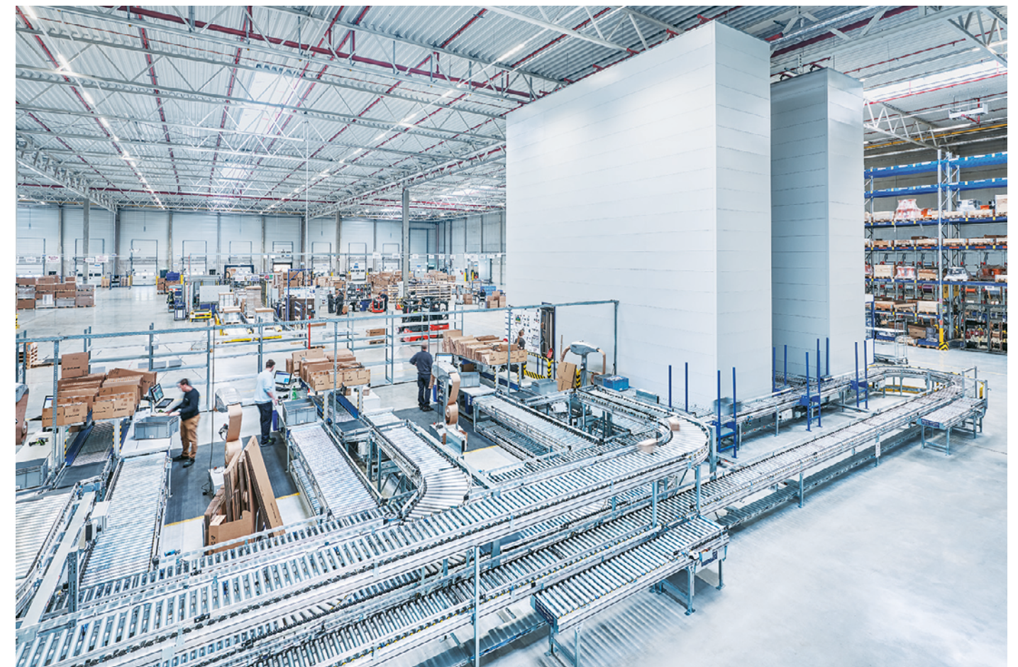
Vertical Buffer Modules Kardex Compact Buffer with automated conveyor connection
